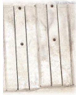
Figure 8. Double coring in the top and middle part of the upper anode.
