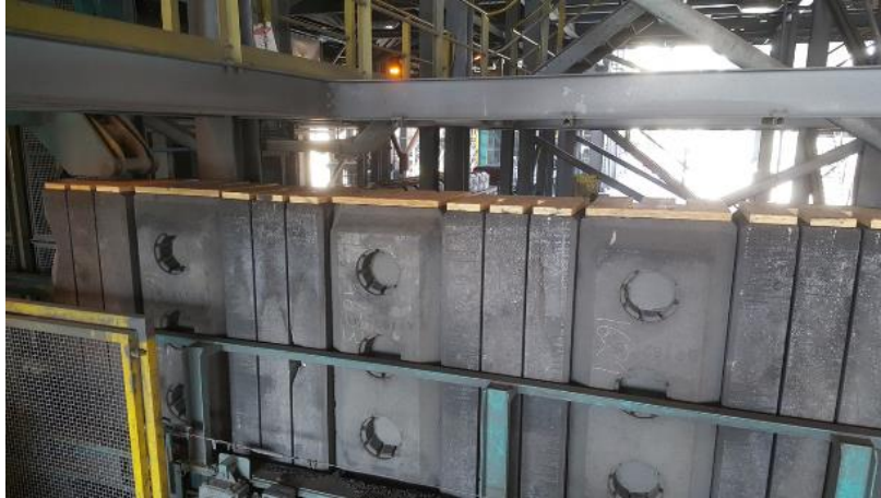
Figure 12. Anodes extended with 20 mm thick wooden plates.
