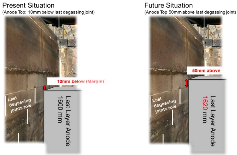
Figure 5. 1620 mm-long anode location vs degassing joint.
