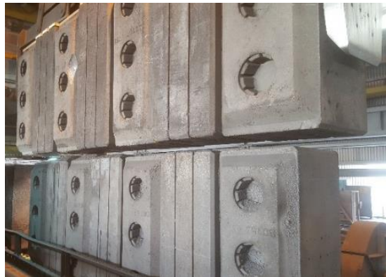
Figure 3. Example of clearance concerns between grabbed and conveyed anode sets.
